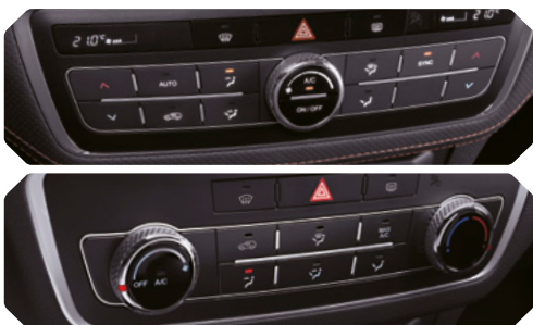
Automatische dual-zone airco / Manuele airconditioning
